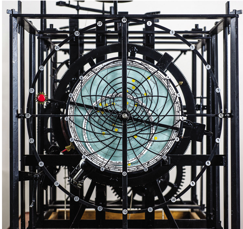
2.9. Principal face of Richard of Wallingford's clock. The unequal hours are the inner circle of numbers from 6 to 6, read on the curves running inwards from them. Note also the sun showing the true solar time, and the golden dragon with its red tongue and tail marking the lunar nodes (1:4 scale reconstruction).
