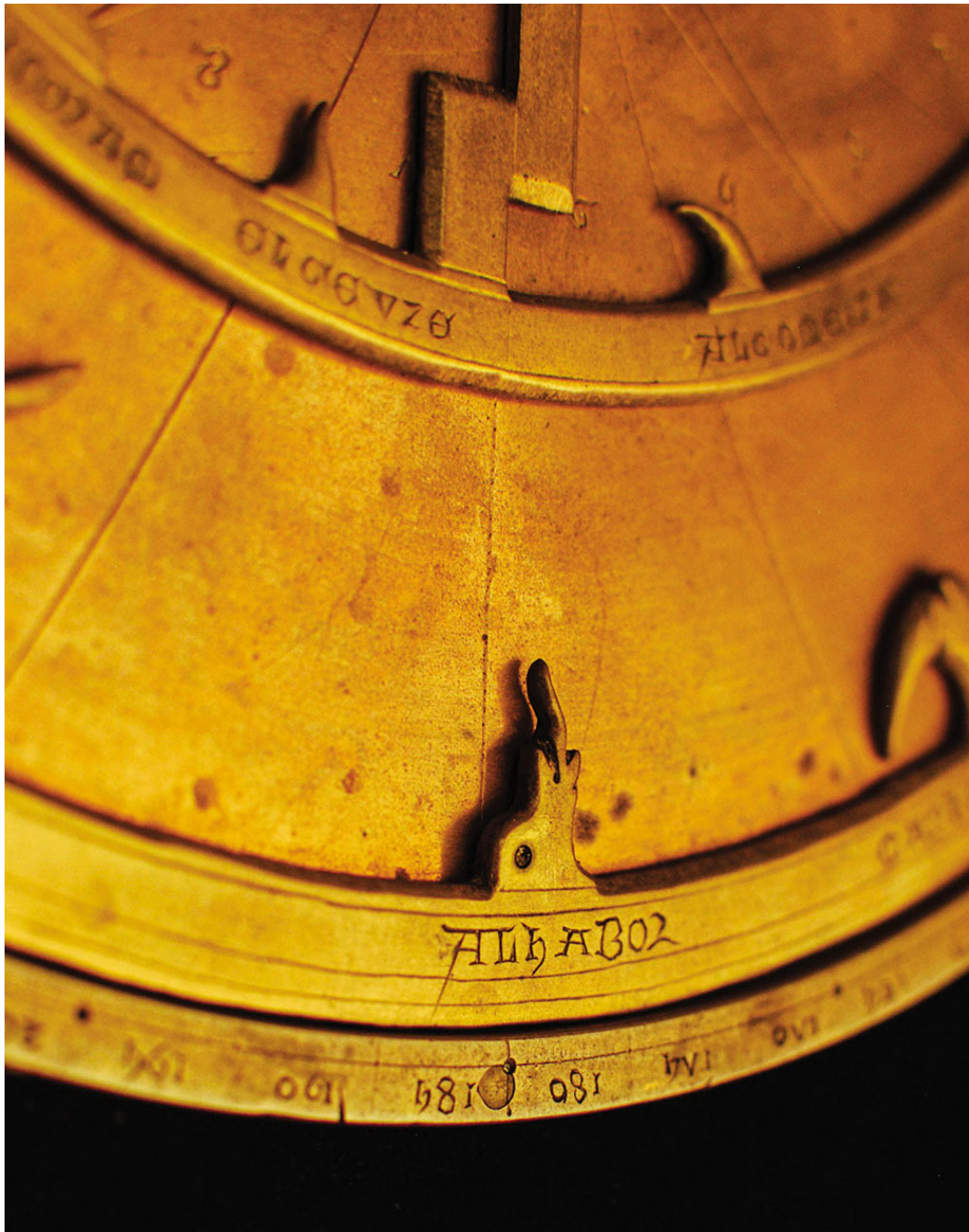
4.9 The head and curving tongue of the dog star, Alhabor (Sirius). The rete here is in place at the bottom of the astrolabe; note the 180-degree marking and twelve o'clock midnight mark on the limb.
